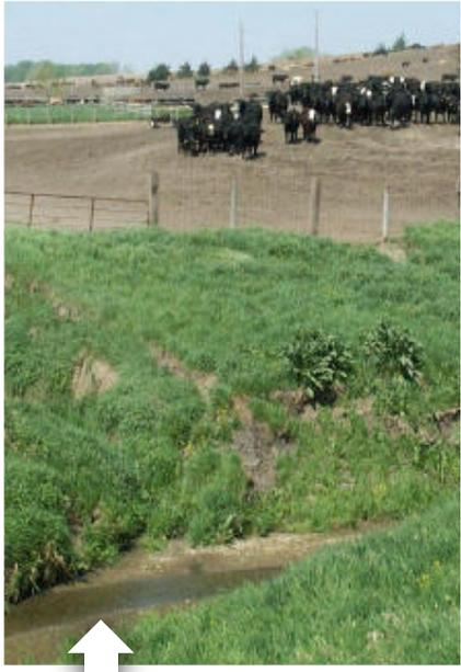
Take the sample in the stream. Pick a location below the pathway(s) where runoff from the lot enters the stream.
