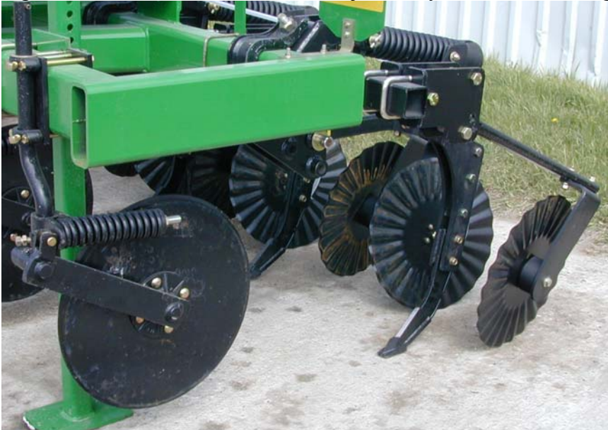
Figure 2. The conventional till knife injection system with covering disks (CTKS).
