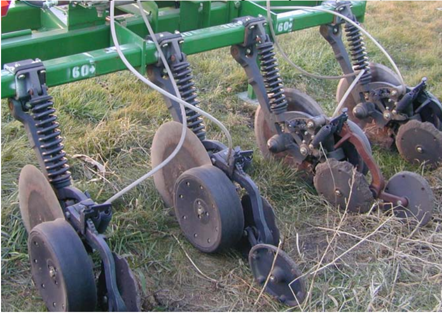
Figure 1. The high speed low draft opener system (HSLD).
