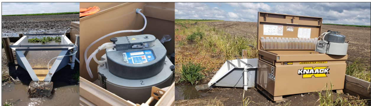
Figure 2. H-flumes and equipment used in the study to measure and sample runoff.
