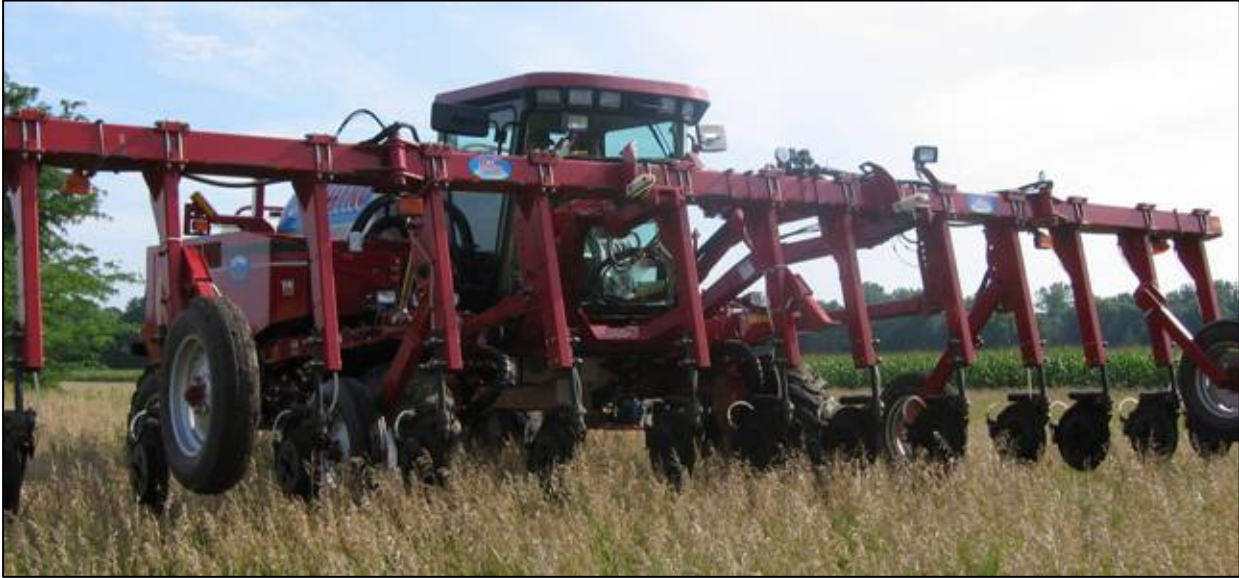
Figure 3. Twelve row-wide, high-clearance applicators and toolbars, used to apply post-sensing N fertilizer at project demonstration sites.
