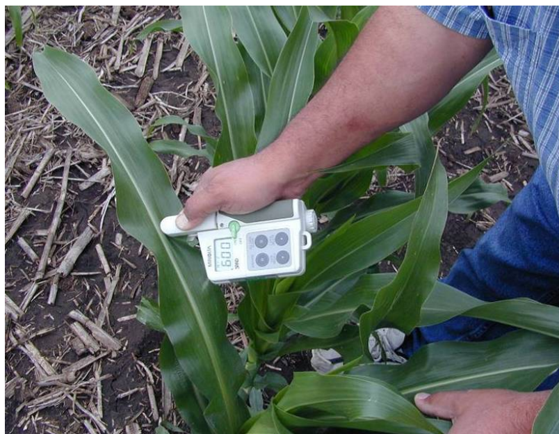
Figure 2. Demonstration of a SPAD chlorophyll meter measuring corn leaf greenness (N status).
