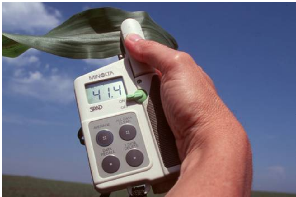
Figure 2. Demonstration of a SPAD chlorophyll meter measuring corn leaf greenness (N status).
