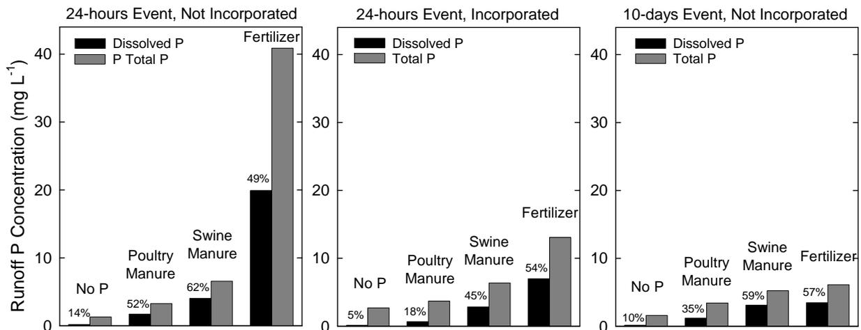
Fig. 4. Dissolved reactive P and total P in runoff as affected by the P source, incorporation, and the timing of a runoff event shortly after applying 100 lb P<sub>2</sub>O<sub>5</sub>/acre. Numbers on top of the bars indicate percent DRP of the total P.
