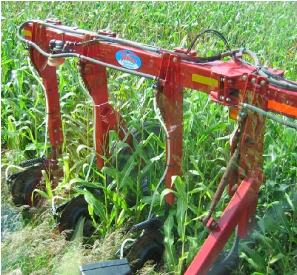
Figure 3. Twelve row-wide, high-clearance nitrogen toolbar used to apply at-tassel N fertilizer in selected N treatment strips at the 2004 Dallas County (Adel) demonstration site on July 21, 2004.
