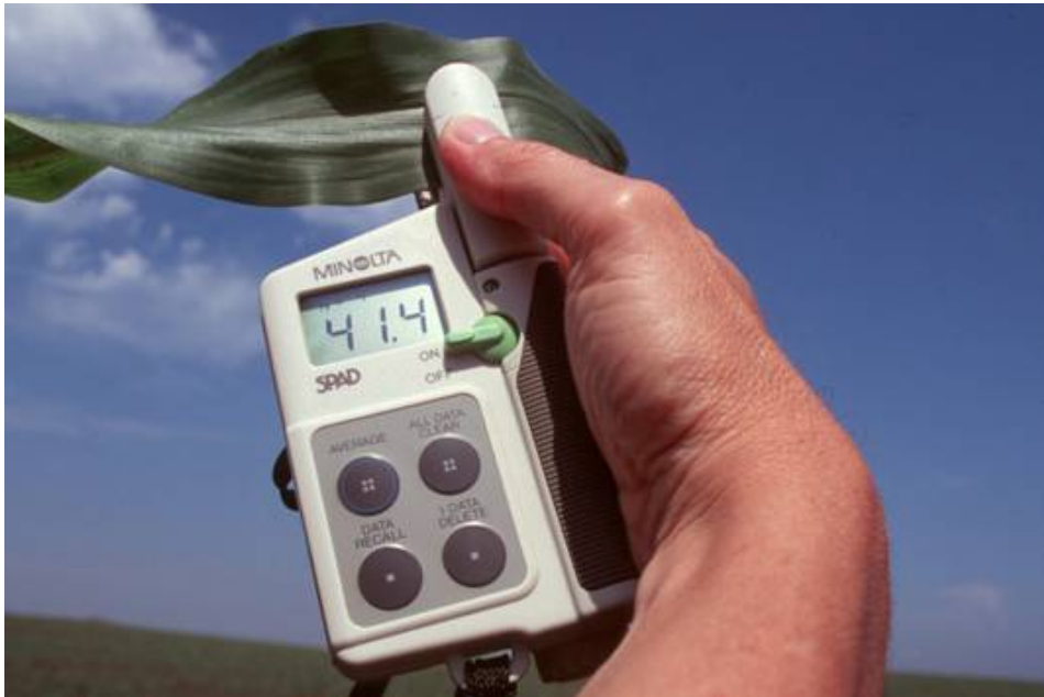
Figure 2. Demonstration of a SPAD chlorophyll meter measuring corn leaf greenness (N status).
