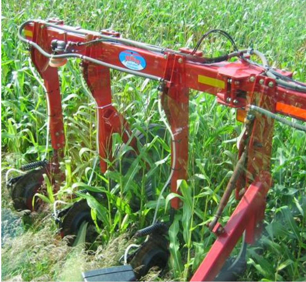
Figure 3. Twelve row-wide, high-clearance nitrogen toolbar used to apply at-tassel N fertilizer in selected N treatment strips at a project demonstration site.
